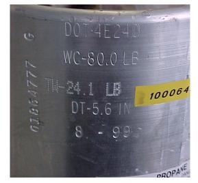
• All DOT Cylinders are required to have an ID stamp embedded in the collar or an ID plate attached. This ID information will identify several important features.
