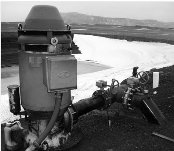
*A variable frequency drive controls the speed of this irrigation pump in Union County, saving electricity.*
