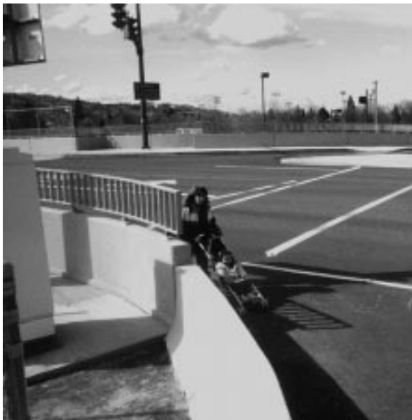
Lack of sidewalk forces pedestrian onto roadway
