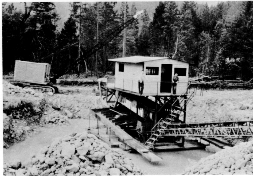
Figure 12-b. Dragline dredge (doodlebug) at the Johnson placer on upper Pleasant Creek, Jackson County, in 1960.
