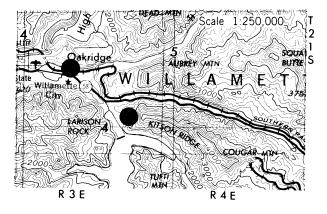
Figure 6. Geothermal drilling, Willamette Pass-Oakridge, 1980. Two holes were drilled in this area by the Oregon Department of Geology and Mineral Industries under the USDOE low-temperature geothermal-resource assessment program. The Oakridge city well was deepened to 1,130 ft, and a 500-ft temperature-gradient well was drilled south of town.
