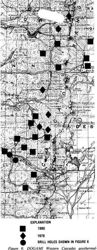
Figure 9. DOGAMI Western Cascades geothermalresource study, 1979-1980. Map shows locations of 500-ft temperature-gradient wells drilled as part of the USDOE geothermal-resource assessment of the Cascades. Also indicated are holes drilled for the low-temperature geothermalresource assessment program (see Figure 6).
