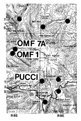
Figure 5. Geothermal drilling in the Mount Hood area, 1980. The Pucci Chairlift hole and unlabeled holes were drilled by the USGS. The Pucci hole was deepened from 2,000 to 4,003 ft. The OMF-1 hole was flow-tested and abandoned by the USDOE. OMF-7A was drilled by the USDOE to 6,027 ft.
