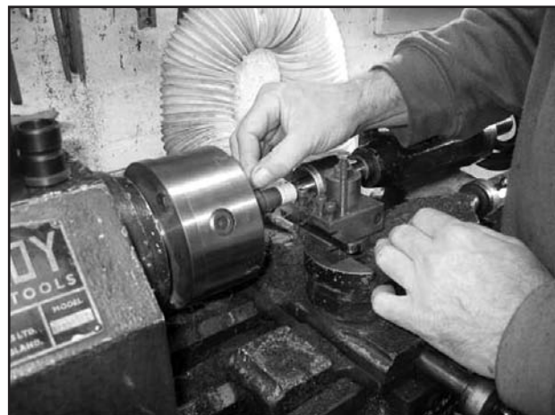
Hazardous exposures are present simply due to the operator's close proximity to the lathe's rotating parts.
