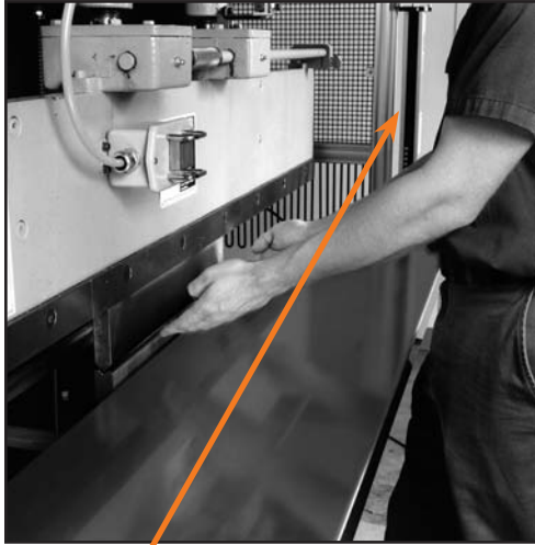
Rockford Systems Inc. Presence-sensing device (light curtain) used.
