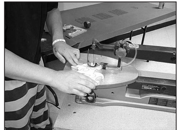
Safety guard/holddown installed.
