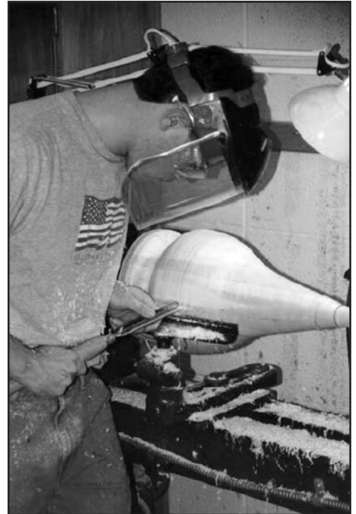
Make sure the tool rest is secure and set close to the stock.
