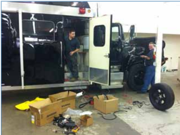
Technicians install the new mobile radio equipment in an Oregon State Police SWAT armored vehicle.
