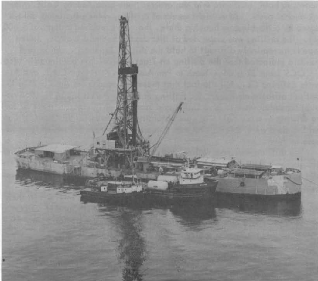
Figure 2. Western Offshore Drilling & Exploration Co. Barge No. III; it was converted from a World War II Navy tanker by Puget Sound Bridge & Dry Dock Co. at Seattle in 1964.
