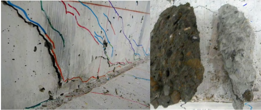
Figure 6.18: Specimen IT.7.18.6.M initial peeling and saturated concrete vs. dry concrete
