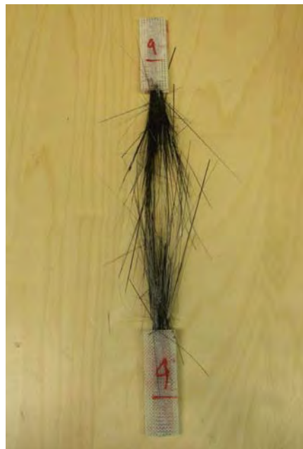
Figure 5.11: Brooming failure of CFRP coupon
