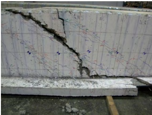
Figure 6.3: Specimen IT.7.18.6.S at failure
