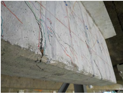
Figure 6.2: Specimen T.6.18.6.S at failure (flexural)
