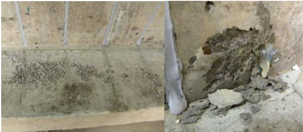
Figure 6.19: Specimen IT.7.22.6.FT effects from freeze-thaw exposure
