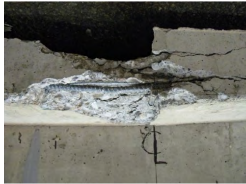
Figure 6.2: Specimen T.6.18.6.S at failure (flexural)
