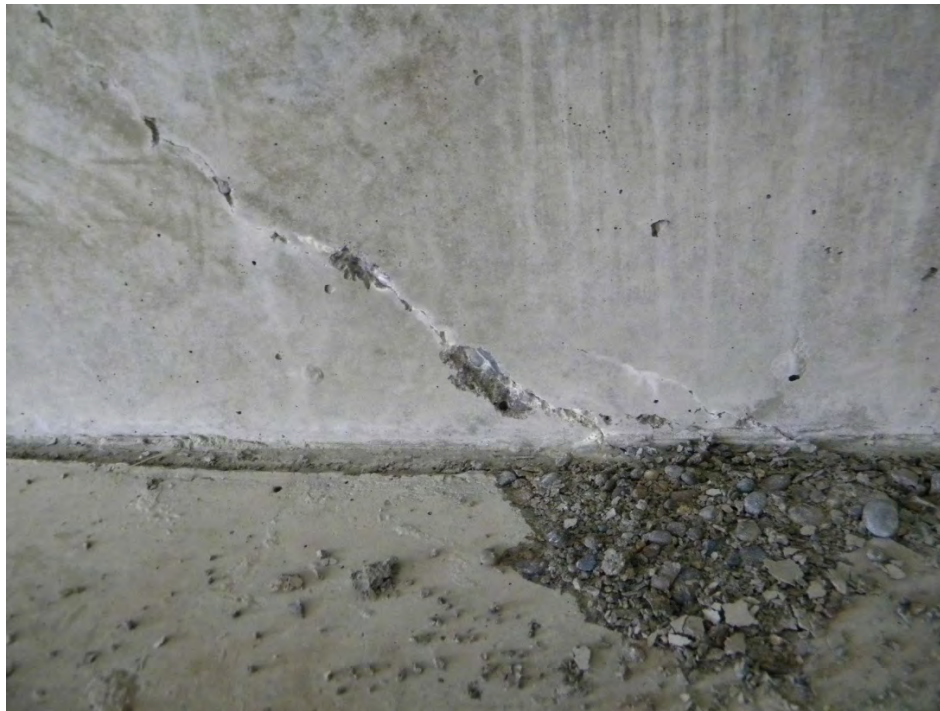
Figure 6.16: Specimen IT.7.22.6.FT/FTG typical raveling along a diagonal crack, scaling of concrete on flange soffit, and associated debris
