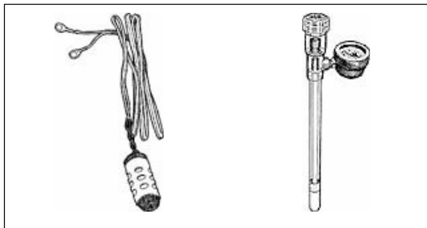
Figure 3. Tensiometer (right), and gypsum block (left), two instruments for monitoring soil moisture levels and scheduling irrigation.
