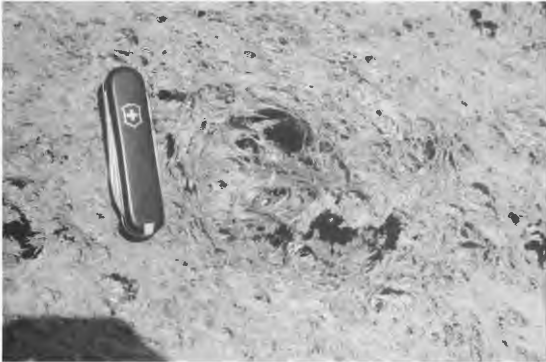
Figure 3. Example of large vesicles in a pumice block from the Mazama (Crater Lake) climactic pumice flow, sample location 14 near Beaver Marsh in Klamath County. Knife is approximately 5 cm long.
