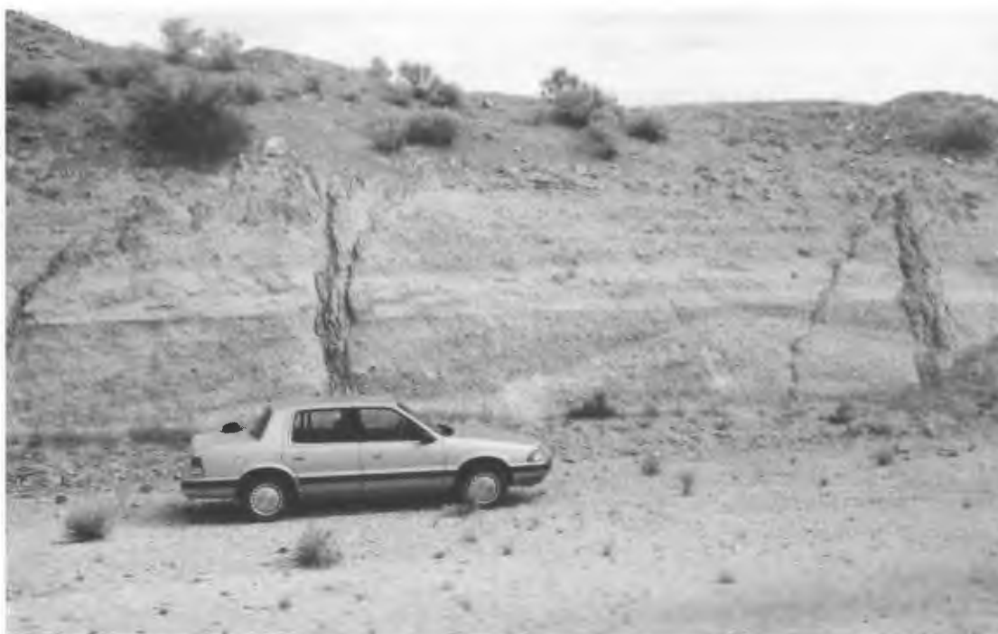
Figure 22. Pumice pit face on Burns Butte, Harney County. This deposit is the result of multiple eruptive events, as indicated by soil horizons, interlayered ash and cinder beds, and abrupt changes in color and induration.
