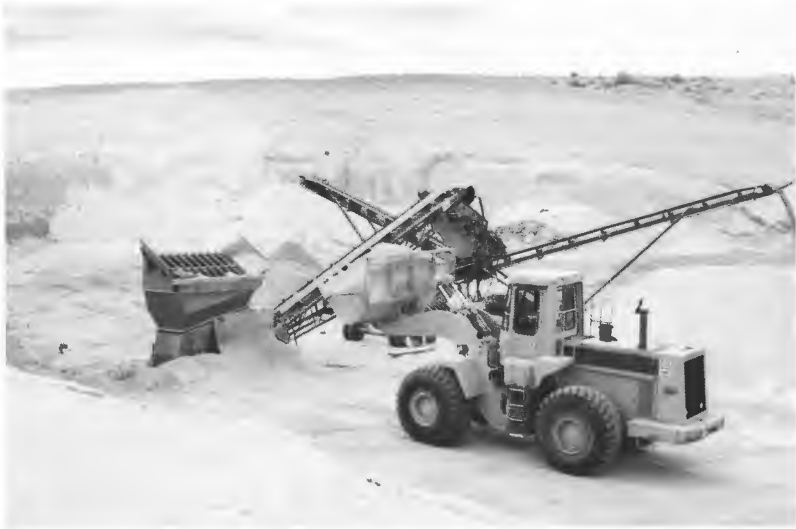
Figure 12. Cascade Pumice Company pit near Tumalo, Deschutes County. Pumice is mined by front-end loader and transported to portable primary crusher and screening plant.
