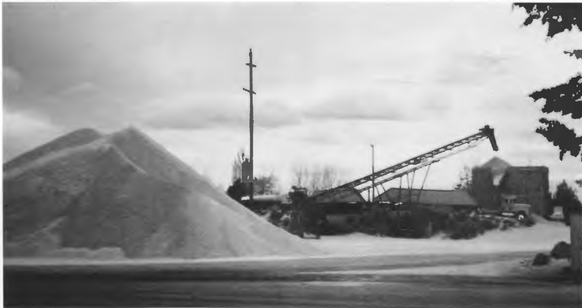
Figure 13. Cascade Pumice Company plant with offloading ore truck, radial stacker, and stockpile.
