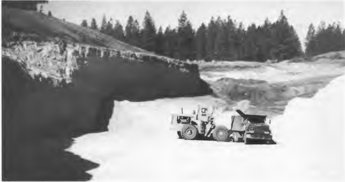
Figure 14. One of several pits of Central Oregon Pumice Company in Bend, Deschutes County. Overburden is removed by bulldozers and scrapers, and pumice is mined by front-end loader.
