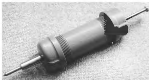
Figure 23. Device built to determine the relative indentation hardness of pumice as measured by the hole diameter produced when the point is supported on a flat surface ground on pumice particles.
